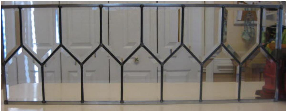
The width is addressed as before. The **smallest height** this layout will fit, using the 9/32" perimeter zinc and the smaller house bevels, is **10 3/4"**. If the opening is under 10 1/2", a house bevel treatment is not possible.
